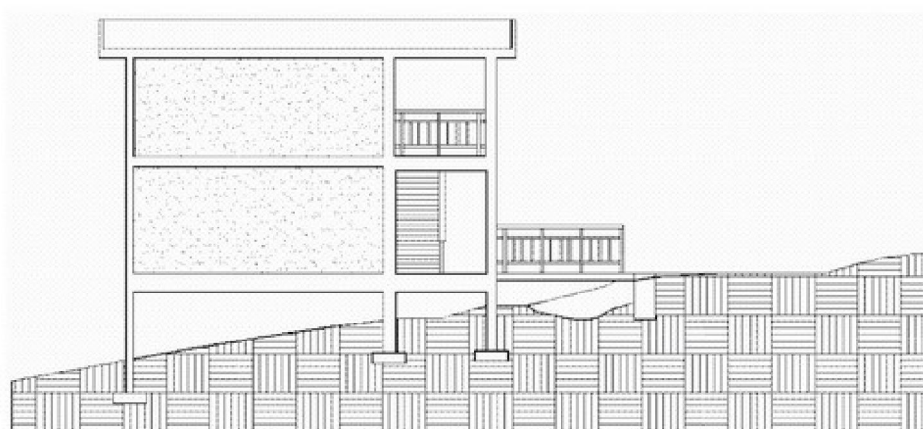
BRIDGES TO PROVIDE ACCESSIBLE ENTRANCES
